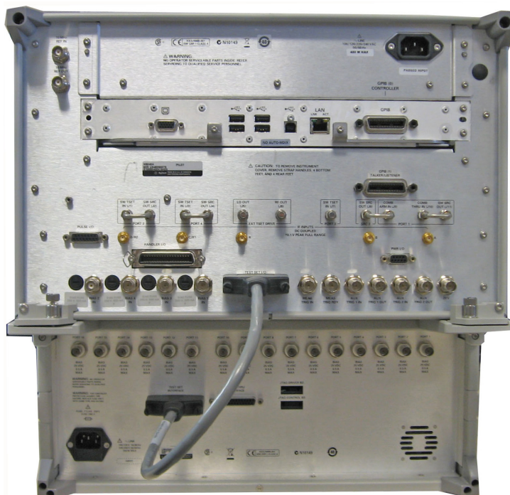
Figure 17 PNA-X Test Set I/O Cable Connection
