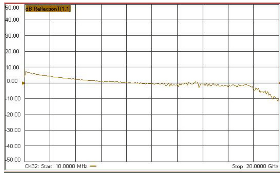
Figure 48 Option 001 or 002 Reflection Tracking Trace (Port 1-8) with PNA-L
